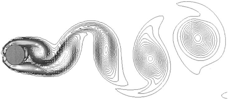
FIG. 8. Vorticity contours for a vortex wake at Re = 200 .
